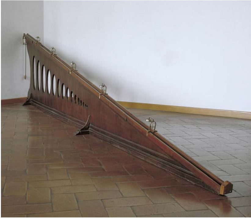
Figure 7: Device of Galileo Galilei for experiments on the law of falling bodies. This device was rebuilt at the Istituto e Museo di Storia della Scienza in Florence. ©Photo Franca Principe, IMSS, Florence.
