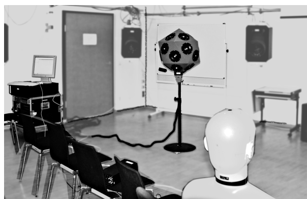
Figure 1. ICO playing spatial music for a dummy listener for the systematic investigation. Exemplary binaural recordings of stimulus 2 are available at: http://iaem.at/Members/zotter/KK_2.wav
