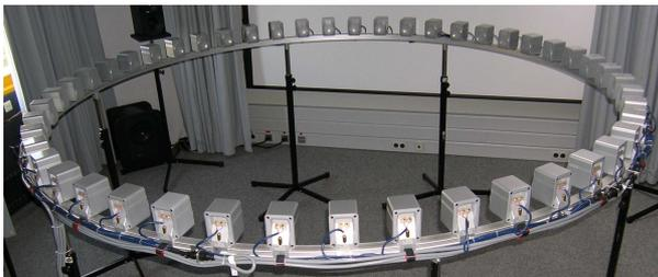
**Figure 1:** 48 channel circular loudspeaker array.
