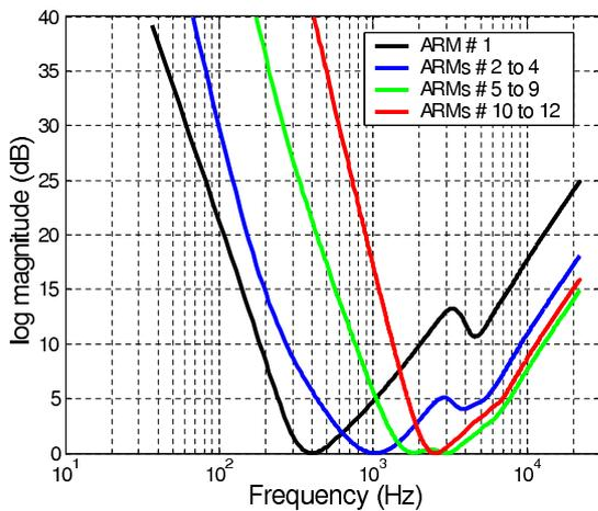
**Figure 8:** Frequency response of sound power equalizers for the ARMs of the spherical array.
