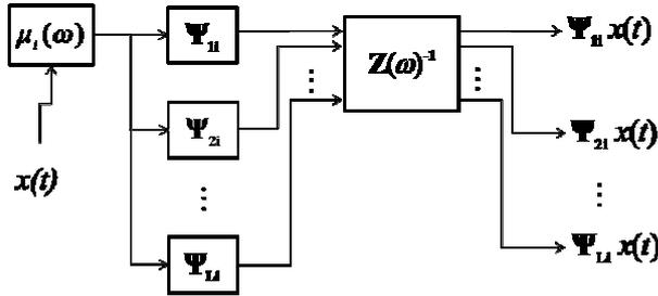
**Figure 3:** Block diagram representing the synthesis of the  $i$ -th ARM of a  $L$ -driver loudspeaker array.
