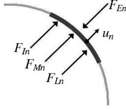
**Figure 2:** Free body diagram of the  $n$ -th spherical cap of the array.
