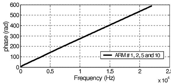
**Figure 10:** Sound pressure response at  $\hat{\mathbf{r}}_p$  for some ARMs of the spherical array with power equalization. IIR equalization filters with  $B = D = 9$ .
