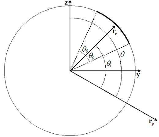
**Figure 1:** Spherical cap with aperture angle  $\theta_0$  mounted on a rigid sphere at  $\mathbf{r}_c$ .
