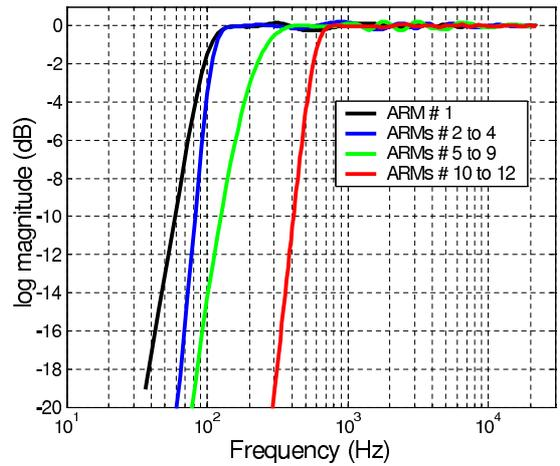
**Figure 9:** Squared sound power response of the power equalized audio system for the ARMs of the spherical array. IIR equalization filters with  $B = D = 9$ .
