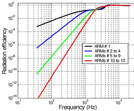
**Figure 7:** Radiation efficiencies of the ARMs of a spherical array with  $a = 0.075\text{m}$ ,  $L = 12$  and  $\theta_0 = 15.86^\circ$ .
