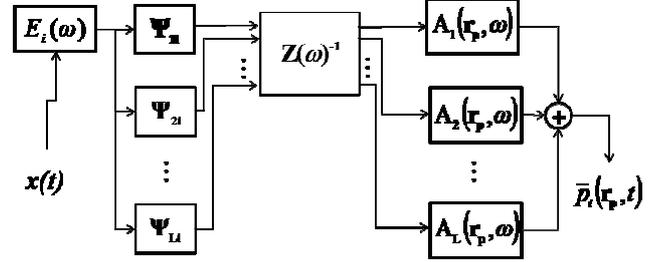
**Figure 4:** Block diagram representing the sound field produced by the  $i$ -th ARM of a  $L$ -driver loudspeaker array after equalization.
