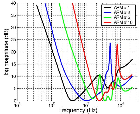
**Figure 6:** Frequency response of sound pressure equalizers for some ARMs of the spherical array.
