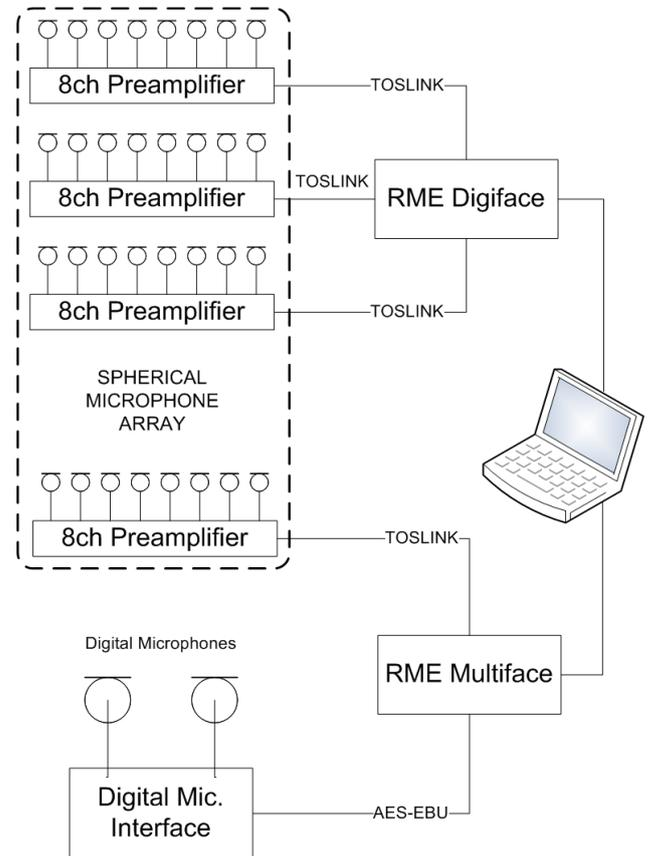
**Figure 3:** Connecting the microphones to the recording device
