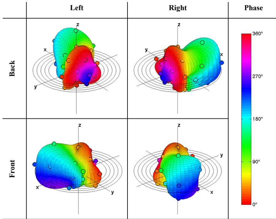
**Figure 7:** Radiated complex sound pressure of the fundamental frequency for a trumpet playing A4 (443 Hz, source assumed to be in the center of the array)
