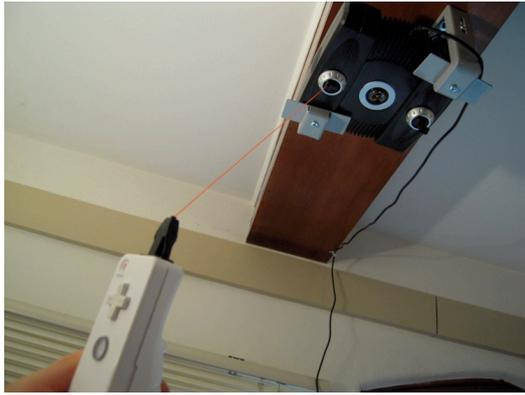
**Figure 9:** 3D position tracking with overhead Gametrak
